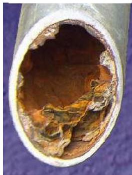
Fig.2: heavily corroded tube in cross section.
