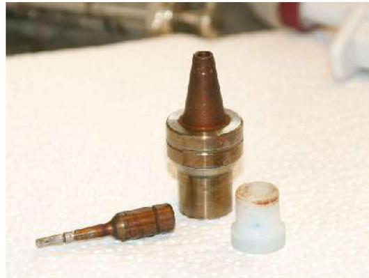
Fig.1: valve of a high pressure pump.
