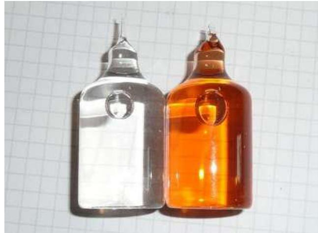
Figure 4: Two vials of an iron rapid-test, filled by a customer at the same sampling point; during the week (left) and on Monday morning (right). The intensity of the color indicates the iron content.
